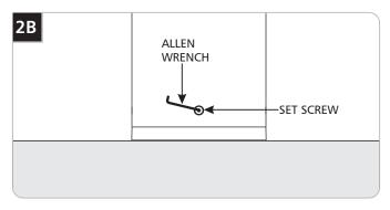
Carefully install the fixture onto the base plate and secure it in place by tightening all set screws.
