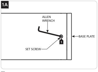
Loosen (Do Not Remove) the set screws on fixture base with the provided Allen wrench and remove the base plate.
