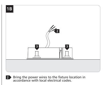
3 Mount the base plate to an even and smooth surface using the provided template on page 4.
